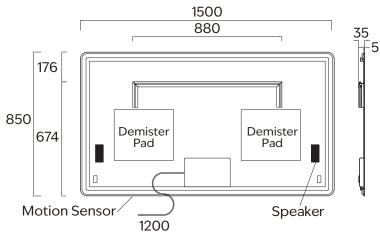
Note: All measurements shown are in millimetres. Sizes are nominal.
