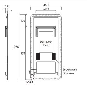
Note: All measurements shown are in millimetres. Sizes are nominal.
